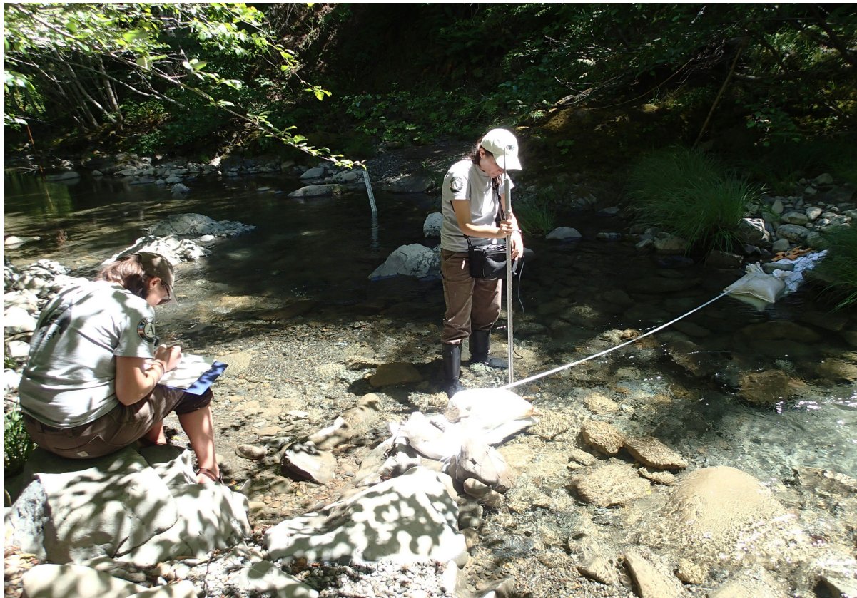
Streamflow monitoring in Mattole Canyon Creek. Photograph courtesy of Sanctuary Forest, Inc.
